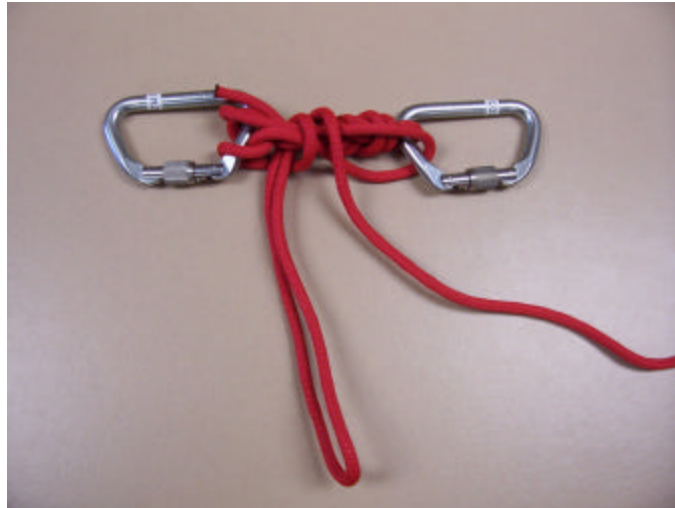
3:1 Radium Release Hitch See Appendix A for step-by-step directions
