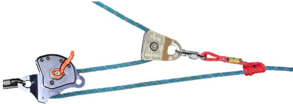
Figure 94- MPD employed in 3:1 simple pulley system.
