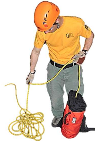
Figure 18- Stacking a rope.
