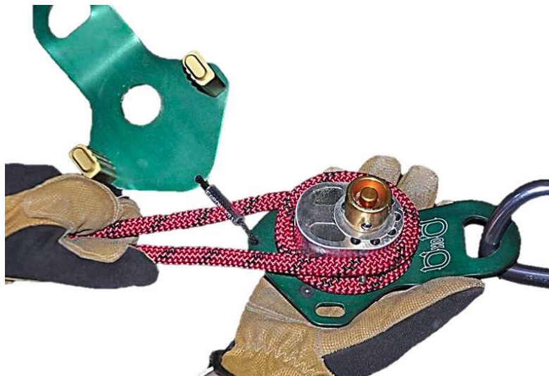
Figure 96- Loading the 540°™ Rescue Belay device with 1 1/2 complete wraps of the rope. The tether cord for the two side plates has been properly positioned between the strands.
