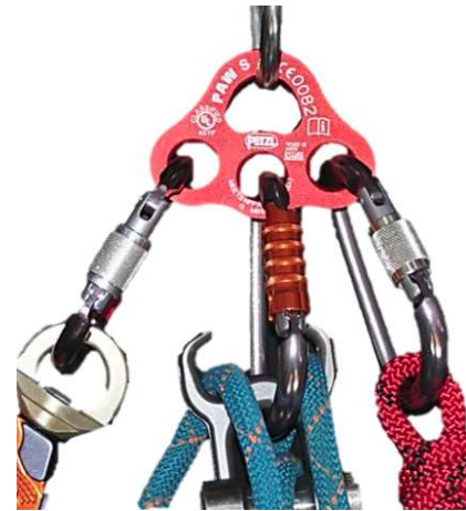
Figure 53- Rigging Plate. Keeps multiple connections organized.
