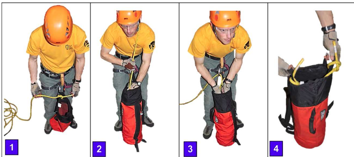
Figure 17- Bagging a rope. 1.) Tie off the initial rope tail to the mouth of the rope bag. 2.) Rope can be directed over the shoulder into the bag. 3.) Alternate technique is to direct the rope through a carabiner on a harness into the bag. 4.) Securing the rope terminus to the mouth of the bag.
