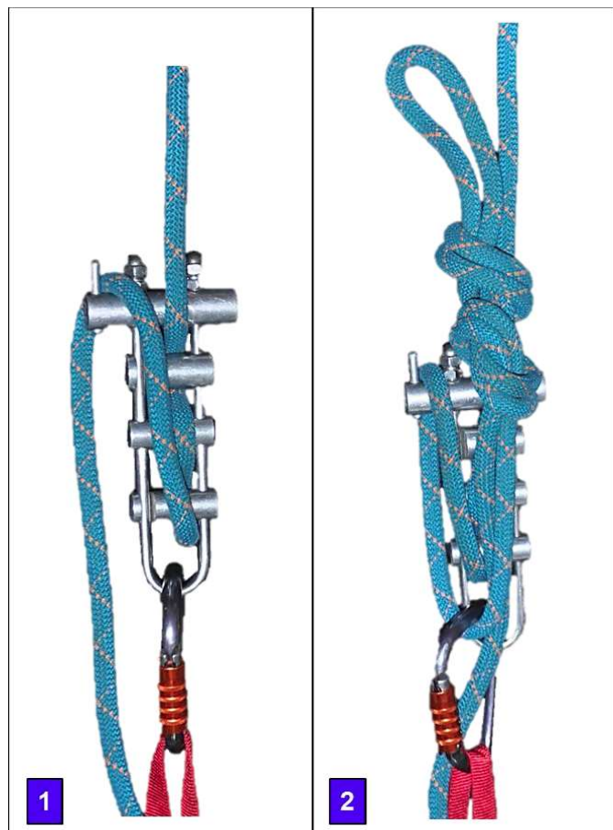
Figure 42- 1.) A quick lock-off of the CMC three-bar rack is achieved with a single Cleat Hitch to one side of the device. 2.) A Cleat Hitch applied to both sides of the device provides an unattended hard tie-off.
