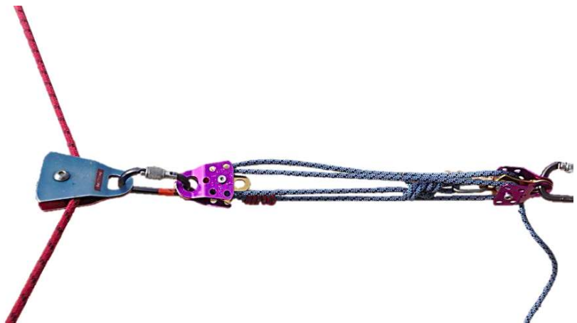
Figure 142- Directional pulley with jigger as adjustable tether.
