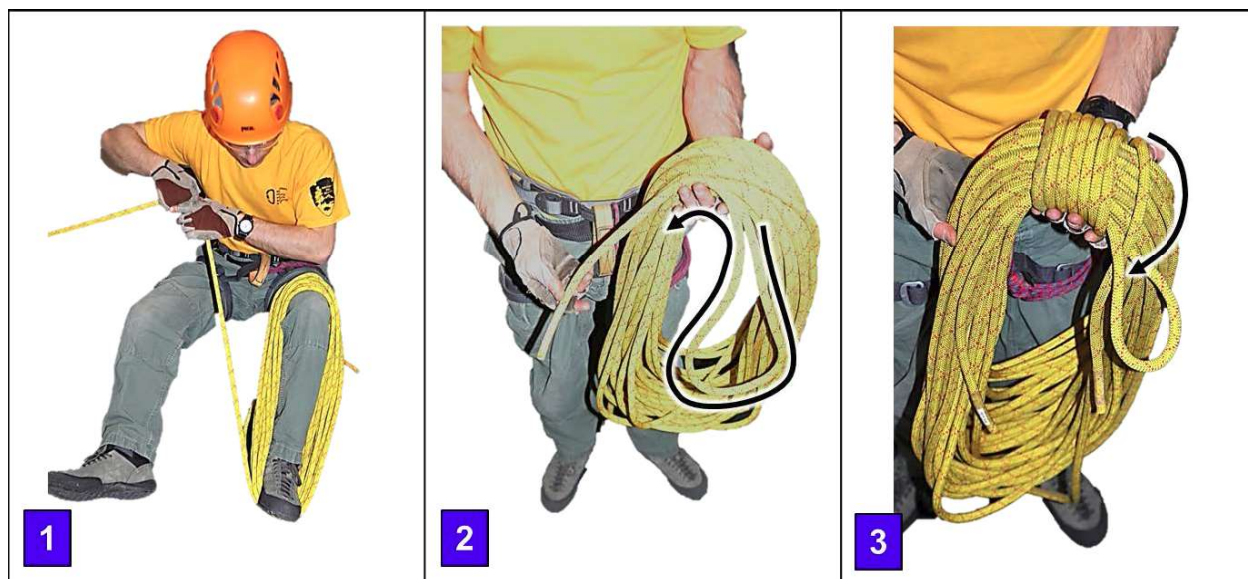
Figure 21- Mountaineer's coil. 1. Form neat equal-sized loops around a leg. 2. Double the rope end back upon itself at the starting end for a 0.6m (2 ft) section. 3. Take the trailing rope end and wrap tightly around the doubled back portion working toward the bight. Finally the terminus of the trailing end is passed through the bight. Pull tight on the opposite tail to secure.
