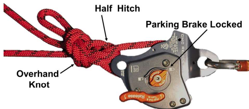
Figure 92- MPD secured with Parking Brake locked and tied off.
