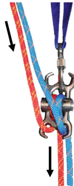
Figure 38- Scarab rigged for a lowering with twin ropes
