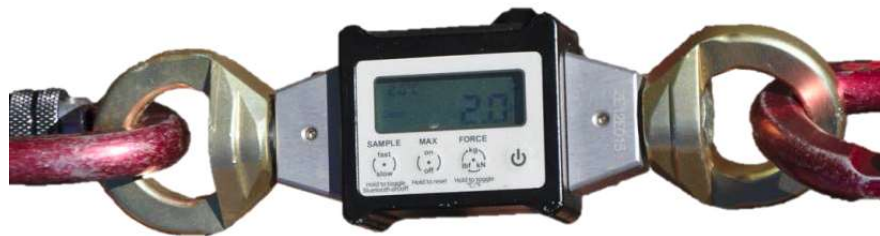
Figure 191- Rock Exotica Enforcer Load Cell
