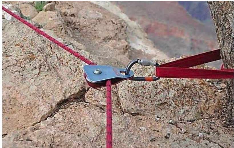
Figure 143- Fixed Directional Pulley
