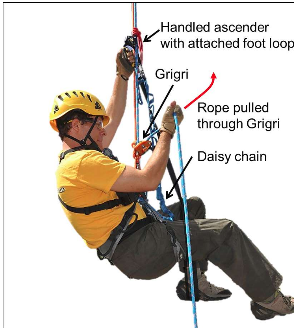
Figure 153- Grigri Ascending Technique
