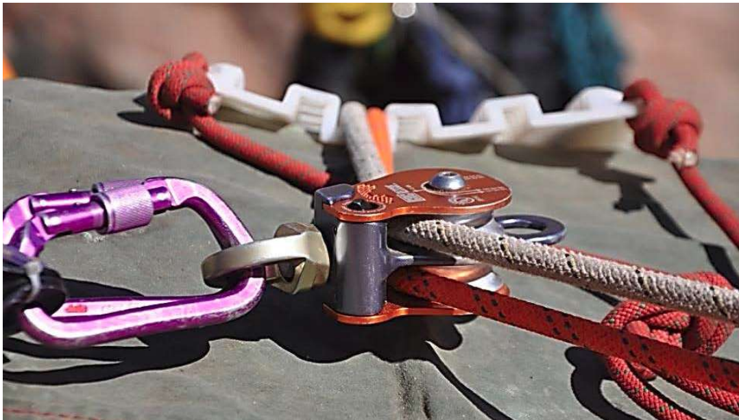
Figure 144- Directional pulley constructed with a double-sheaved swivel pulley (Rock Exotica Omni-Block Double) to provide alignment of both the main line and belay line.
