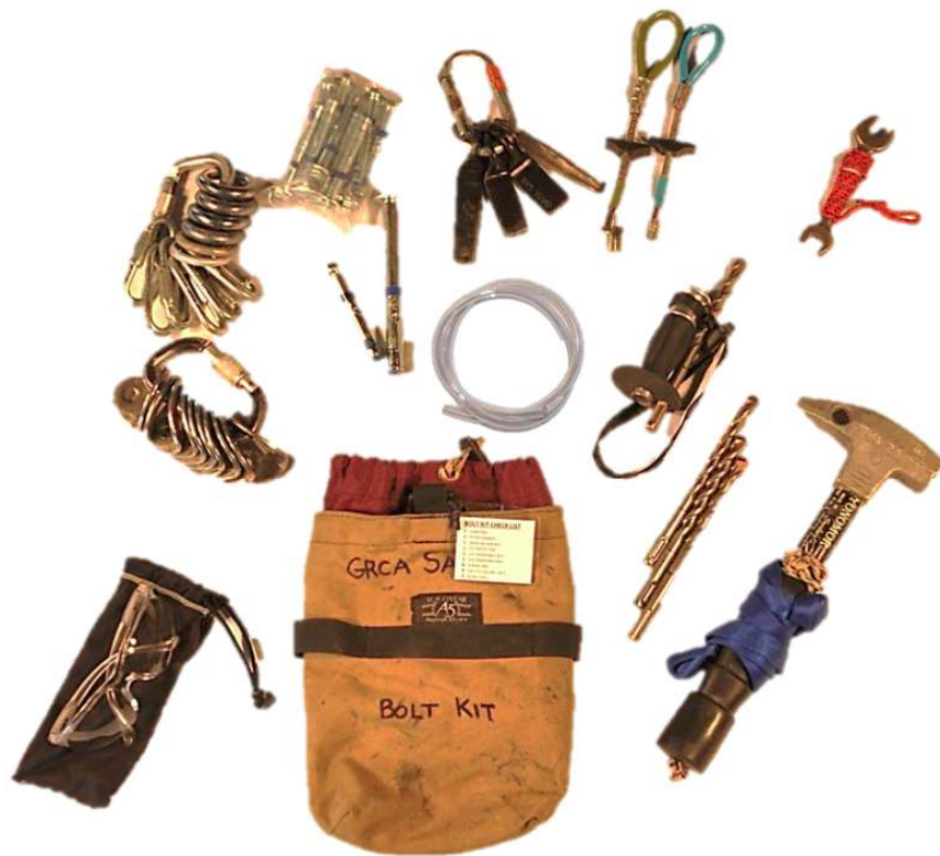
Figure 130- Bolt Kit. Contents clockwise from top; pitons, blow tube, removable bolts, wrench, hand drill, spare SDS bits, rock hammer, storage bag, safety glasses, bolt hangers, rappel rings, and expansion bolts.
