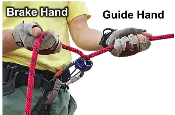
Figure 85- Belaying method technique typically employed by recreational climbers, with device attached to the belayer's harness.
