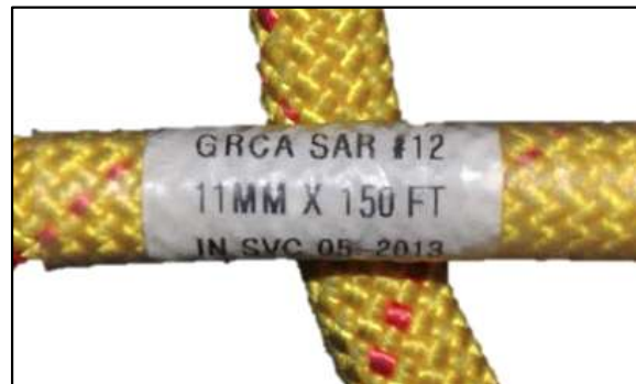
Figure 15- Rope label. Provides identification number, diameter, length and in service date.
